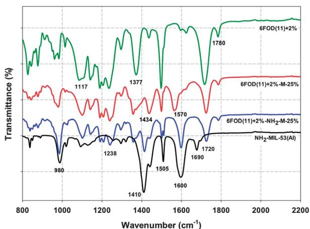
**Fig. 8** ATR-FTIR spectra between 800 and 2200 cm<sup>-1</sup> for NH<sub>2</sub>-MIL-53(Al), 6FOD(11) + 2% and their MMMs (all spectra are shifted upward by 2.5, 5.0, and 7.5%, respectively, except NH<sub>2</sub>-MIL-53(Al)).
