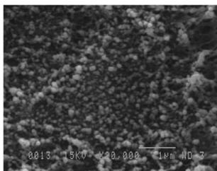
Fig. 6 SEM micrograph of 6FOD(11) + 2% with 15 wt% MIL-53(Al).
