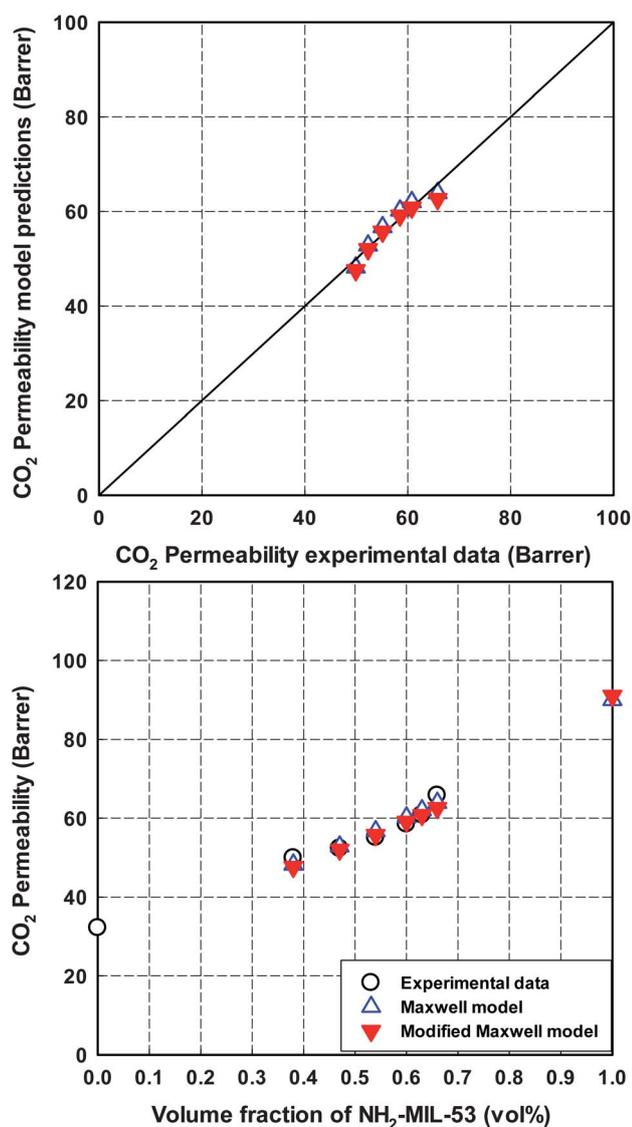
**Fig. 15** Comparison of CO<sub>2</sub> permeability of 6FOD(11) + 2%-NH<sub>2</sub>-MIL-53(Al) MMMs between experimental data and predictions from the Maxwell model and the modified Maxwell model. The optimized CH<sub>4</sub> permeability of pure NH<sub>2</sub>-MIL-53(Al) is predicted by the Maxwell model.
