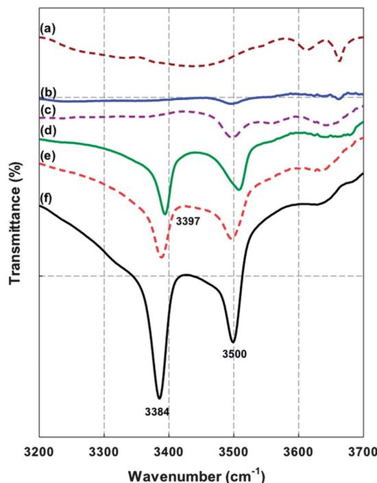
**Fig. 9** ATR-FTIR spectra between 3200 and 3700 cm<sup>-1</sup> for (a) MIL-53(Al); (b) 6FOD(11) + 2%-M-25%; (c) 6FOD(11) + 2%; (d) 6FOD(11) + 2%-NH<sub>2</sub>-M-15%; (e) 6FOD(11) + 2%-NH<sub>2</sub>-M-25%; and (f) NH<sub>2</sub>-MIL-53(Al) membranes (all spectra are shifted upward by 25, 50, 75, 100, and 125%, respectively, except NH<sub>2</sub>-MIL-53(Al)).
