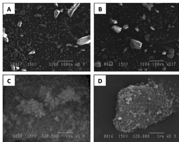
Fig. 1 SEM photo of MIL-53(Al) (A and C) and NH<sub>2</sub>-MIL-53(Al) (B and D).
