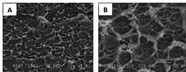
**Fig. 3** SEM micrographs of (A) Matrimid 5218 membrane with 15 wt% NH<sub>2</sub>-MIL-53(Al); (B) Ultem 1000 membrane with 15 wt% NH<sub>2</sub>-MIL-53(Al).
