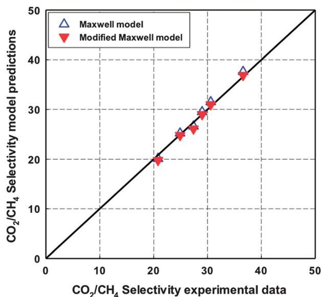
**Fig. 16** Comparison of CO<sub>2</sub>/CH<sub>4</sub> ideal selectivity of 6FOD(11) + 2%-NH<sub>2</sub>-MIL-53(Al) MMMs between experimental data and predictions from the Maxwell model and the modified Maxwell model.
