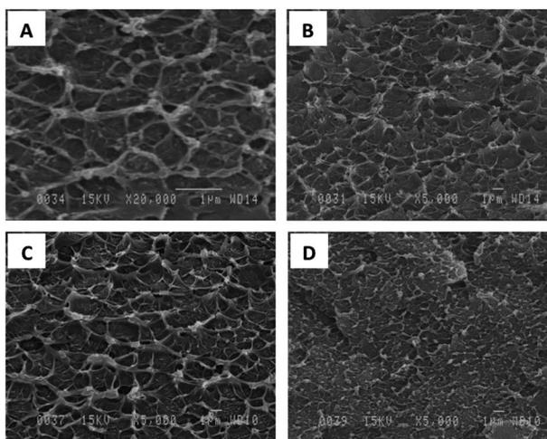
**Fig. 5** SEM micrographs of 6FOD(11) + 2% with (A) 20 wt%; (B) 25 wt%; (C) 30 wt%; and (D) 35 wt% of NH<sub>2</sub>-MIL-53(Al).
