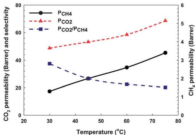
**Fig. 13** CO<sub>2</sub> and CH<sub>4</sub> permeability and ideal selectivity of 6FOD(11) + 2%-NH<sub>2</sub>-M-30% membrane as a function of temperature. The lines are general trends.
