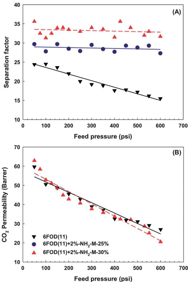
**Fig. 12** Comparison between (A) separation factor and (B) CO<sub>2</sub> permeability of neat polyimide and co-polyimide-MOF MMMs for gas blends. The lines are general trends.
