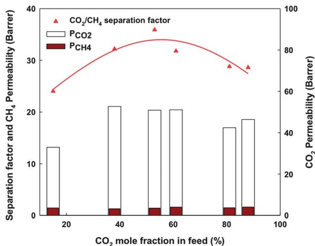
**Fig. 14** Separation factor, permeability of CO<sub>2</sub> and CH<sub>4</sub> in gas blends as a function of CO<sub>2</sub> mole fraction in feed.
