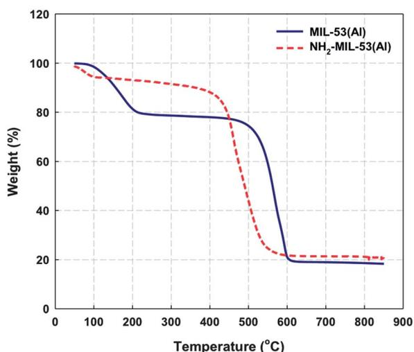
**Fig. 2** TGA curves of non- and amino-functionalized MIL-53(Al).
