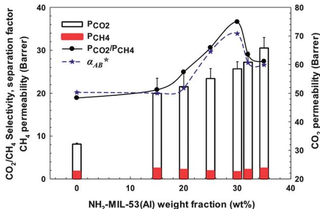
**Fig. 11** CO<sub>2</sub> and CH<sub>4</sub> permeabilities, ideal selectivity ( $P_{CO_2}/P_{CH_4}$ ) and separation factor ( $\alpha^*$ ) for CO<sub>2</sub>:CH<sub>4</sub> = 50:50 as a function of NH<sub>2</sub>-MIL-53(Al) loading at 308K and 150 psi for 6FOD(11) + 2%-MOF MMMs.
