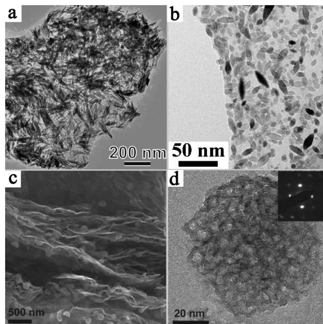
**Fig. 8** Several types of TiO<sub>2</sub> nanostructures on graphene. (a) Rutile TiO<sub>2</sub>/graphene. Reprinted with permission from ref. 128. Copyright 2010 American Chemical Society; (b) TiO<sub>2</sub> nanospindles/graphene oxide. Reprinted with permission from ref. 129. Copyright 2010 American Chemical Society; (c) and (d) mesoporous anatase TiO<sub>2</sub>/graphene. Reprinted from ref. 130 with permission by Wiley-VCH.
