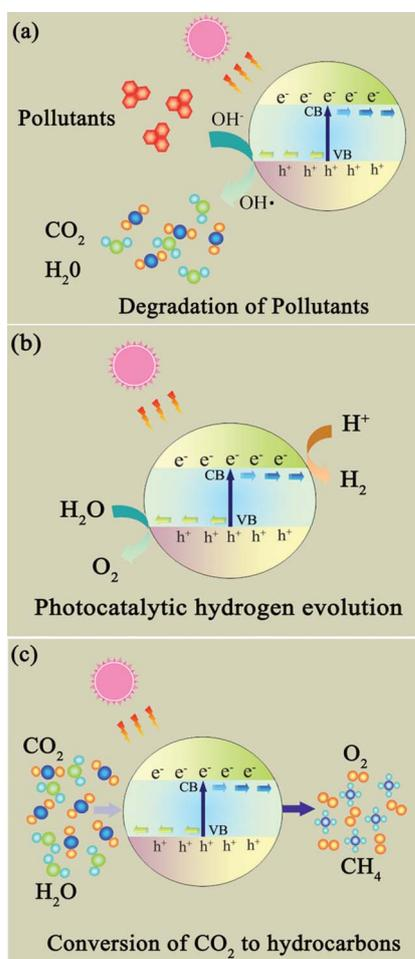
**Fig. 6** The photocatalytic applications of photocatalysts. (a) Degradation of organic pollutants; (b) photocatalytic hydrogen generation; (c) photocatalytic conversion of CO<sub>2</sub> to hydrocarbon fuels.
