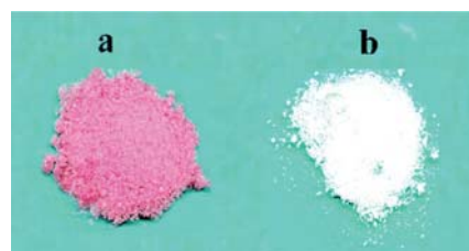
Fig. 2 Picture of poly(methyl methacrylate) (PMMA) synthesised by the RAFT process (a) before and (b) after reaction with AIBN. 45
