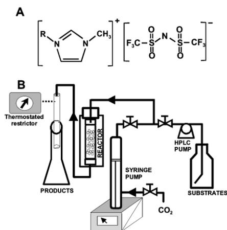
**Fig. 1** A. Structure of 1-alkyl-3-methylimidazolium triflimide, obtained according to Lozano *et al.*<sup>7</sup> B. Experimental set-up.
