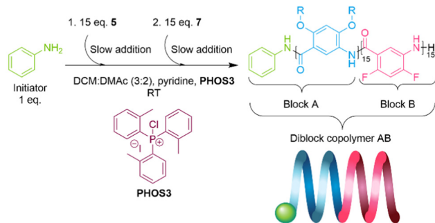
Scheme 2 Top: Synthetic paths for monomers 5 and 7 . (a) K_2CO_3 , DMF, 15-bromo-2,5,8,11-tetraoxapentadecane 2 , 51%. (b) H_2/Pd/C , MeOH, EtOAc, quant. (c) KOH, EtOH, 60%. (d) H_2/Pd/C , MeOH, EtOAc, quant. Bottom: Polymerization conditions of diblock copolymer AB.
