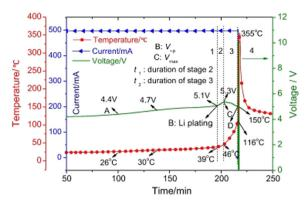
Fig. 13 Stages of overcharge induced thermal runaway based on overcharging experiments combined with ARC. Reproduced with permission from ref. 240. Copyright 2016, Elsevier Ltd.
