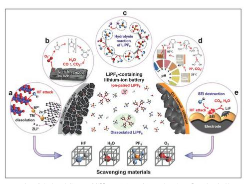
Fig. 10 Schematic representation of the key challenges of LiPF<sub>6</sub>-containing carbonate electrolytes. Reproduced with permission from ref. 217. Copyright Wiley-VCH: (a) transition metal dissolution resulting from HF attack, (b) gas evolution triggered by solvent decomposition, (c) hydrolysis reaction of LiPF<sub>6</sub> to form HF and corrosive acids, (d) thermal decomposition of LiPF<sub>6</sub>, (e) interfacial layer destruction by HF attack.
