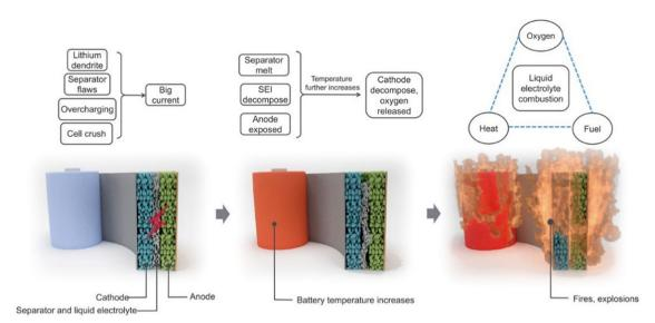
gas release process Fig. 1 The stages of thermal runaway in LIBs. Reproduced with permission from ref. 11. Copyright 2018, American Association for the Advancement of Science
