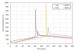
Fig. 15 Comparison of surface temperatures during ARC tests. Reproduced with permission from ref. 262. Copyright 2020, Elsevier B.V.
