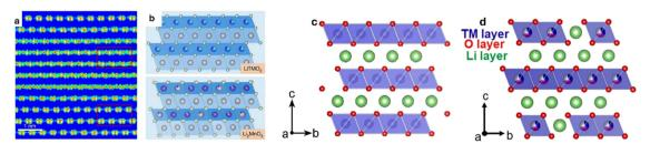
Fig. 2 (a) High-resolution TEM image, and (b) schematic structure of LiTMO<sub>2</sub> and Li<sub>2</sub>MnO<sub>3</sub> domains. Reproduced with permission from ref. 51. Copyright 2024, The Author(s). Licensed under Creative Commons CC BY(https://creativecommons.org/licenses/by/4.0/). Structures of (c) Ni-rich layered oxide, (d) and Li-rich layered oxide. Reproduced with permission from ref. 52. Copyright 2021, Elsevier B.V.
