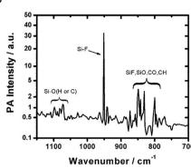
Fig. 7 (a) The main degradation mechanisms of Si anode. Reproduced from ref. 174. Copyright 2016, Macmillan Publishers Limited. (b) Photoacoustic infrared spectroscopy of the interfacial layer formed on Si-anode surface from unwanted reaction with LiPF<sub>6</sub>-based carbonate electrolyte. Reproduced with permission from ref. 173. Copyright 2014, The Royal Society of Chemistry.
