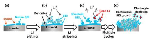
Fig. 9 Schematic diagram showing (from left to right) (a) pristine Li metal with heterogeneous native SEI layer, (b) growth of Li dendrites during Li plating, (c) loss of Li<sup>+</sup> ("dead Li") and growth of residual SEI during Li stripping, and (d) continuous SEI growth and electrolyte depletion after multiple plating/stripping cycles. Reproduced under the terms of the ACS AuthorChoice License.<sup>130</sup> Copyright 2020, American Chemical Society.
