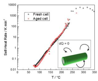
Fig. 26 Thermal abuse ARC experiments under quasi-adiabatic conditions. Reproduced with permission from ref. 362. Copyright 2017, Elsevier
