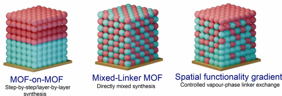
Scheme 1 A schematic illustration of mixed-linker MOF structures with different possible spatial configurations and fabrication methods; left to right: MOF-on-MOF, homogeneously mixed-linker and the spatial gradient, which is demonstrated in the current work. Two differently colored spheres are used to represent different linker's presence in the MOF.
