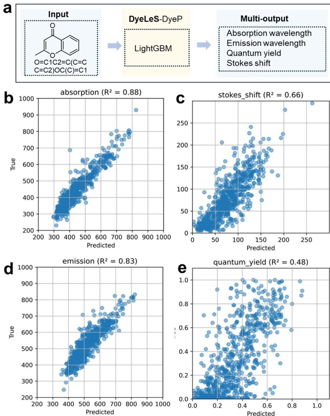
**Fig. 4** Workflow and performance of DyeLeS-DyeP. (a) Workflow of DyeLeS-DyeP: molecular structures are input into a multivariate regression model, which outputs predictions for (b) absorption wavelength, (c) Stokes shift, (d) emission wavelength, and (e) fluorescence quantum yield. The corresponding  $R^2$  values are 0.88, 0.66, 0.83, and 0.48, respectively.
