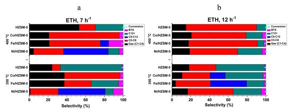
Fig. 2 (a) and (b) Product distribution and ethanol conversion in the ETH process.
