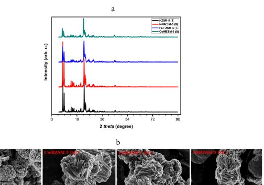
Fig. 7 (a) XRD pattern and (b) SEM images of spent catalysts (operating condition: 350  $^{\circ}$ C and 7 h<sup>-1</sup>).
