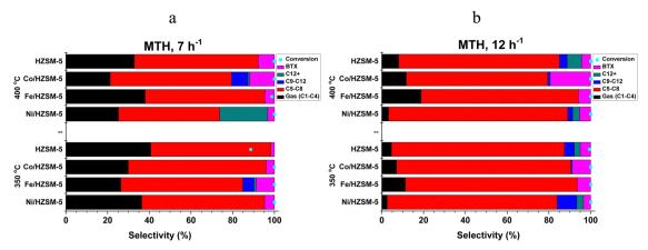
Fig. 1 (a) and (b) Product distribution and methanol conversion in the MTH process.
