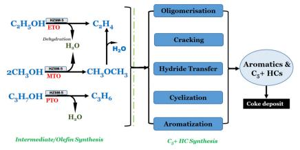
Reaction pathway for the conversion of low alcohols (methanol, ethanol and propanol) to hydrocarbons.
