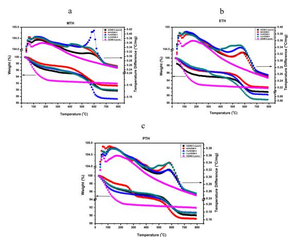
Fig. 6 TGA-DTA profile of (a) MTH, (b) ETH and (c) PTH conversion at  $T=350~{\rm ^{\circ}C}$  and WHSV = 7 h $^{-1}$ .
