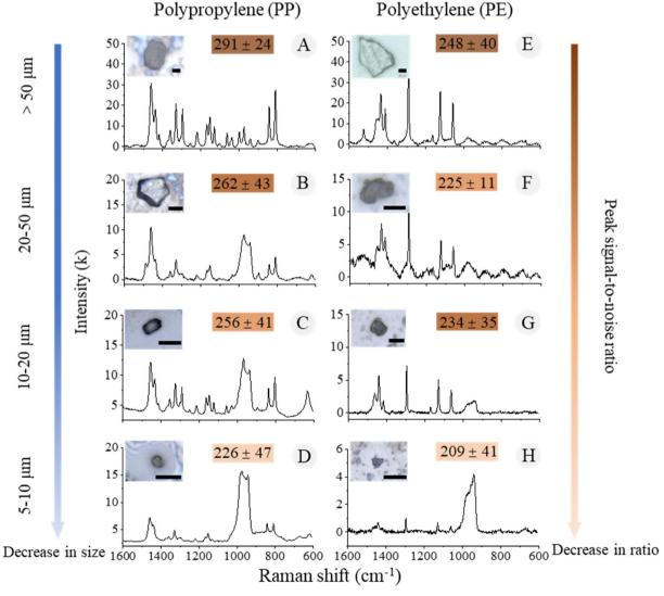
Fig. 4 The morphological and chemical information of MPs in different size fractions. (A–D) PP particles; (E–H) PE particles. Scale bar = 20 μm.
