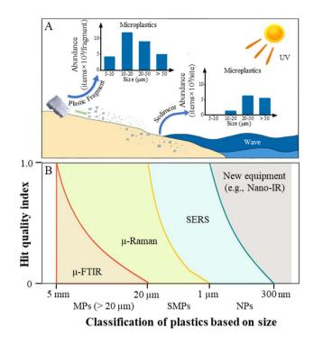
Fig. 8 Underestimation of MPs and limit of analysis methods. (A) Abundance of MPs/NPs from sediment and plastic pieces; (B) hit quality index (HQI) of three identification methods for different sizes of particles.
