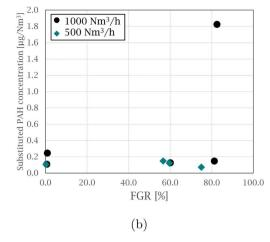
Fig. 6 Graphs showing the estimated PAH stack emissions for PAH-42 and substituted PAHs (sum of oxy- and nitro-PAHs) for both 1000 Nm $^3$  h $^{-1}$  and 500 Nm $^3$  h $^{-1}$  at varying FGR levels. (a) PAH-42 and (b) substituted PAH.
