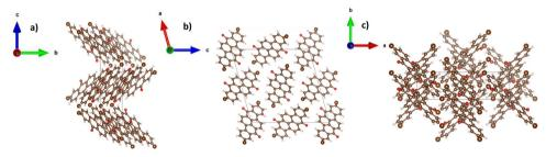
Fig. 9 Crystal structure of vat orange 1, with the view from (a) a-axis, (b) b-axis and (c) c-axis.
