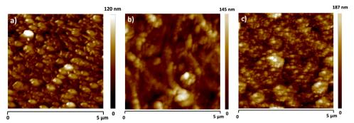
Fig. 6 Atomic force microscopy (AFM) images of 80 nm deposited thick film of the vat orange dyes: (a) vat orange 1 (rms  $\sim$  12.5 nm), (b) vat orange 3 (rms  $\sim$  15.1 nm) and (c) vat orange 9 (rms  $\sim$  20.4 nm).
