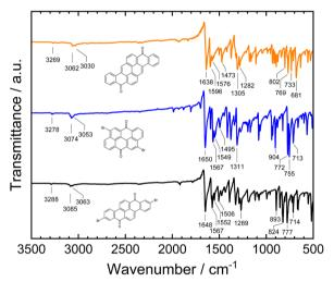
**Fig. 4** FTIR spectra of the purified powders of vat orange 1 (black), vat orange 3 (blue) and vat orange 9 (orange). The labels in the graph indicate the wavenumber positions of selected bands (in cm<sup>-1</sup>).
