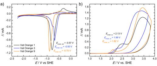
Fig. 3 Cyclic voltammetry (CV) scans of the (a) reductions and (b) oxidations of vat orange 1 (black line), vat orange 3 (blue line) and vat orange 9 (orange line). The samples were used as thin films deposited by thermal evaporation on ITO/glass substrates. Scans were performed at a scan rate of 20 mV s<sup>-1</sup> in a 0.1 M TBAPF<sub>6</sub> solution in acetonitrile.
