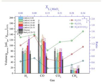
Fig. 5 Total volume of the gaseous products from pyrolytic processes of the LMO-G,  $MnO_2$ -G and glucose samples, all normalized per gram of glucose (bottom and left axes), as well as  $H_2$  and carbon oxide ratios obtained as a function of molar ratio (top and right axes).
