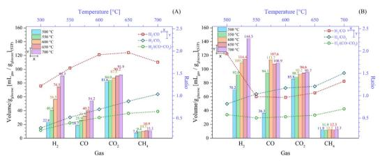
Fig. 7 Total volume of the gaseous products from dynamic-isothermal process (bottom and left axes) of the LMO-G 25-75 sample between 500 °C and 700 °C after the heating dynamic steps (A) and after the whole process (B), all normalized per gram of glucose. Corresponding  $H_2$  and carbon oxide ratios are presented as a function of the target temperature (top and right axes).
