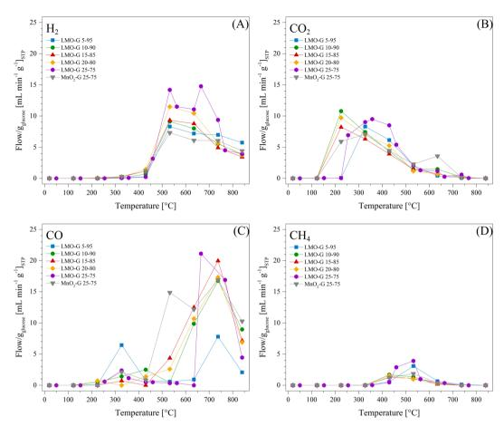
Fig. 4 Thermal evolution of the produced gases ((A)  $H_2$ , (B)  $CO_2$ , (C) CO and (D)  $CH_4$ ) for LMO-G and MnO<sub>2</sub>-G samples, from 30 °C to 850 °C in  $N_2$ , at a heating rate of 30 °C min<sup>-1</sup>. All samples normalized per gram of glucose.
