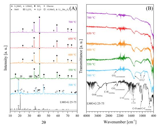
Fig. 8 XRD patterns of the solid products of dynamic-isothermal processes using LMO-G 25-75 (A) and respective ATR-FTIR spectra (B), where LMO-G sample is included for comparison.
