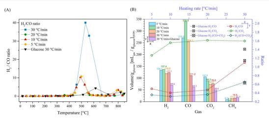
Fig. 3 H<sub>2</sub>/CO ratio evolution from 30 °C to 850 °C for LMO-G 25-75 and glucose samples at different heating rates (A). Total volume of the gaseous products (B) from the corresponding pyrolytic processes, normalized per gram of glucose (bottom and left axes) and the respective H2: CO<sub>x</sub> ratios as a function of the heating rate (top and right axes).
