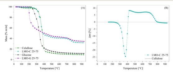
Fig. 9 Thermogravimetric analyses of the cellulose mixture with or without  $\text{Li}_2\text{MnO}_3$  at 30 °C min<sup>-1</sup> in  $\text{N}_2$  flow (A). Normalized weight loss percentages to cellulose content (B) compared with cellulose pyrolysis alone (black line at zero position). Glucose and LMO-G 25-75 results are added in the panel (A) for comparison.
