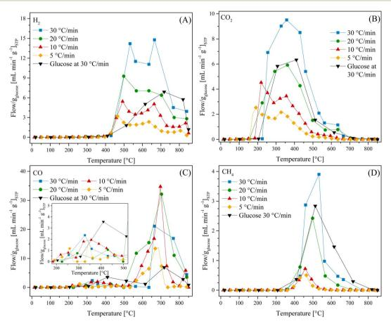
Fig. 2 Thermal evolution of different gases ( $H_2$  (A),  $CO_2$  (B), CO (C) and  $CH_4$  (D)) for LMO-G 25-75 and glucose samples from 30 °C to 850 °C using different heating rates (5, 10, 20 and 30 °C min<sup>-1</sup>), all normalized per gram of glucose.
