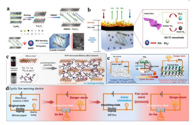
Fig. 25 (a) Synthetic scheme for HDBAC- $Ti_3C_2T_x$  and PLA/HD-TC/SiAPP. (b) Flame-retardant mechanism, reproduced from ref. 373 with permission from Elsevier, copyright 2022. (c) Low-temperature assembly for PVP-decorated MXene paper. (d) MXene paper-based firedetecting sensing device (schematic). (e) Resistance transition mechanism of a C/N-doped TiO2 network, reproduced from ref. 374 with permission from Elsevier, copyright 2022.
