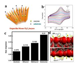
Fig. 17 (a) Encapsulation of haemoglobin in an organ-like MXene. (b) CV results of a Nafion/Hb/Ti<sub>3</sub>C<sub>2</sub>/GC electrode, reproduced from ref. 267 with permission from IOP Science, copyright 2015. (c) Different terminations on MXene nanosheets. (d) Average sensing response for various gases, reproduced from ref. 269 with permission from American Chemical Society, copyright 2017.
