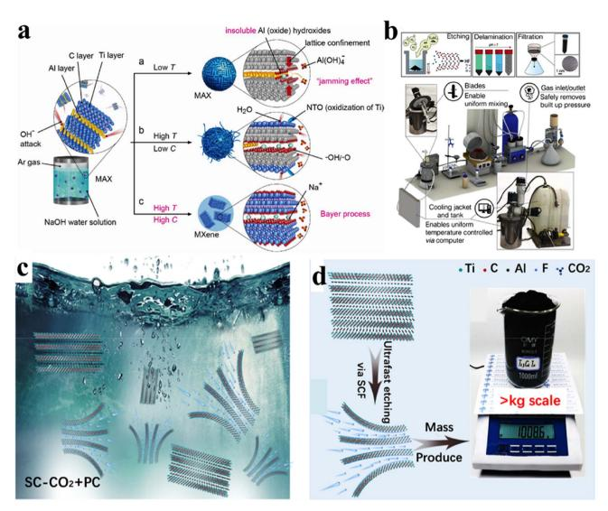
Fig. 5 (a) Representation of hydrothermal synthesis, reproduced from ref. 103 with permission from Wiley, copyright 2018. (b) Synthesis of MXene via a scalable approach, reproduced from ref. 67 with permission from Wiley, copyright 2020. (c) Large-scale synthesis of MXenes via immersion of  $Ti_3AlC_2$  in PC solution. (d) Etching via SCF and obtained  $Ti_3C_2T_x$  in kilogramme-scale, reproduced from ref. 109 with permission from Elsevier, copyright 2023.
