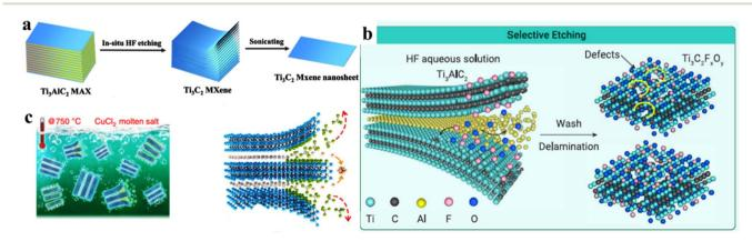
Fig. 3 Synthetic schemes of MXene. (a)  $Ti_3C_2$  MXene nanosheets by *in situ* HF etching, reproduced from ref. 75 with permission from Springer Nature, copyright, 2021. (b)  $Ti_3C_2$  MXene nanosheets by HF etching, reproduced from ref. 82 with permission from ScienceDirect, copyright, 2023. (c) Development of a MXene by molten salt, reproduced from ref. 89 with permission from *Nature*, copyright, 2020.
