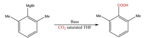
Scheme 9 2,6-Dimethylphenylmagnesium bromide carboxylation at room temperature, using different bases and THF saturated in CO<sub>2</sub>. A maximum yield of 77% is obtained after 30 min using DBU (1,8-diazabicycloundec-7-ene) 50 mol%.<sup>74</sup>
