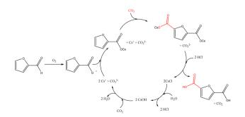
Scheme 14 Overview of the reaction steps for the conversion of furfural to FDCA using the carboxylation route.<sup>65</sup>
