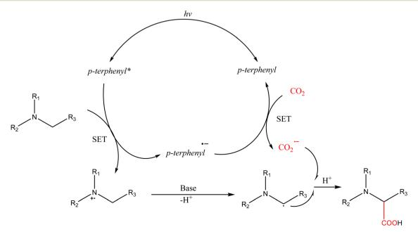
Scheme 6 Photocatalytic  $\alpha$ -carboxylation of amines with CO<sub>2</sub> in continuous flow<sup>41</sup> (SET = single-electron transfer).
