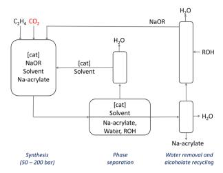
Scheme 13 : Process concept for the Pd-catalyzed synthesis of sodium acrylate from ethylene and  ${\rm Co_2}$  using amide solvents and  ${\rm NaO}$ - $i{\rm Pr.^{107}}$
