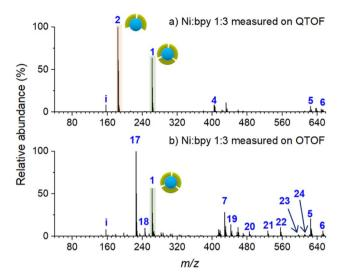
Fig. 1 ESI-MS of solutions prepared by mixing  $NiSO_4$  and bpy in a 1:3 molar ratio measured on the (a) QTOF (harsher conditions) and (b) OTOF (softer conditions) instruments. The pictograms symbolize the number of ligands coordinated to Ni. Green symbols represent the bpy ligand.
