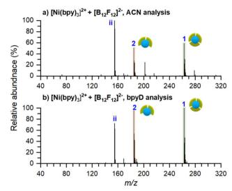
Fig. 5 Ex situ MS of the co-deposition experiments of  $[Ni(bpy)_3]^{2^+}$  with  $[B_{12}F_{12}]^{2^-}$  measured with (a) ACN and (b) 3  $\mu$ M bpyD in ACN as the nano-DESI solvent. The pictograms symbolize the number of ligands coordinated to Ni. Green symbols represent bpy. No species containing bpyD are observed in panel (b). Peaks originating from the solvent are not marked in the spectra for simplicity.
