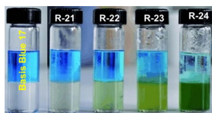
Fig. 6 Visualization of the \text{Cl}^- extraction by the receptors R-21 to R-24 using Basic Blue 17 (top layer: aqueous solution, bottom layer: \text{CH}_2\text{Cl}_2 ). (Reproduced with permission from ref. 51. Copyright 2018, Wiley.)
