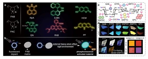
Fig. 7 (a) Structures of the polymers (PAB and PAC) and the dopants: NpA, S-BN, HCM, QN, RhB and PF. (b) Illustration of the general strategy. (c) Structures of the aromatic sodium carboxylates and SA. (d) Luminescence photographs of single-component-doped, co-doped, and TS-FRET SA films with multicolor and multi-tunable afterglows. Reproduced with permission from (a and b) ref. 107 (copyright 2021, John Wiley and Sons) and (c and d) ref. 108 (copyright 2022, John Wiley and Sons).
