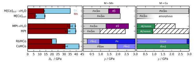
Fig. 2 (Left) Bulk moduli of various PBAs where the values for the Cu-based and Mn-based PBAs are indicated in blue and red, respectively. Note that the bulk modulus of RbMnCo(CN)<sub>6</sub> is calculated based on solely two data points. (Right) The phase diagrams of Cu- and Mn-based PBAs where hashed bars denote unsolved phases. The data for the Mn-PBAs are taken from ref. 31, 37 and 50.
