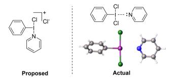
Fig. 6 (Left) Proposed structure of the active intermediate for interaction of PhICl<sub>2</sub> and pyridine. (Right) Actual structure of the intermediate confirmed by X-ray diffraction.
