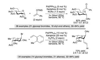
Scheme 28 Visible light-induced, Pd-catalyzed couplings of acetylated glycosyl bromides with silyl enol ethers and styrene derivatives.
