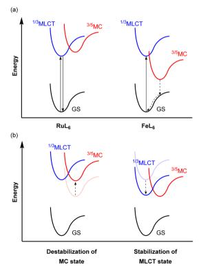
Fig. 21 (a) Simplified potential energy surface diagrams of six-coordinate Ru(II) and Fe(II) complexes. (b) Strategies to achieve a larger energy barrier between MLCT and MC states.
