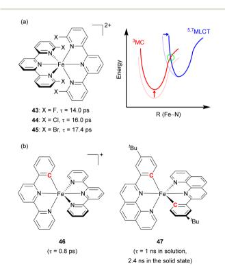
Fig. 22 (a) Structures of Fe( $\parallel$ ) complexes with halogen-substituted terpyridine and the energy levels of MLCT and MC states. (b) Structures of cyclometalated Fe( $\parallel$ ) complexes.
