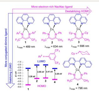
Fig. 2 Summary of heteroleptic Cu(N^N)(NacNac<sup>R</sup>) complexes and their frontier orbital energy levels. Frontier orbital energies were determined by DFT.
