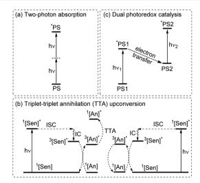
Fig. 6 Summary of strategies for achieving longer wavelengths in the activation of photoreactions through multiphoton absorption. (a) Two-photon absorption. (b) Dual photoredox catalysis. (c) Triplettriplet annihilation upconversion. (PS = photosensitizer, Sen = sensitizer, An = annihilator, ISC = intersystem crossing, and IC = internal conversion, and PS1 and PS2 can be the same or different photosensitizers)
