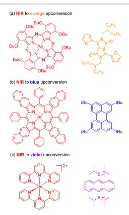
Fig. 8 The control of output light via changing the sensitizers and annihilators. (a) NIR to orange upconversion. (b) NIR to blue upconversion. (c) NIR to violet upconversion.
