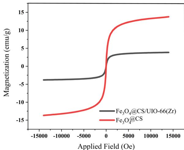
Fig. 9 VSM magnetization of  $\text{Fe}_3\text{O}_4@CS$  and  $\text{Fe}_3\text{O}_4@CS/UIO-66-NH_2(Zr)$ .
