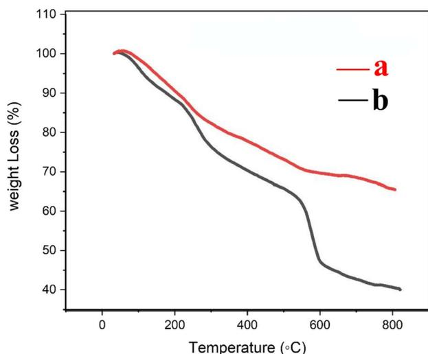
Fig. 6 TG curves (a) Fe<sub>3</sub>O<sub>4</sub>@CS/UIO-66-NH<sub>2</sub>(Zr) and (b) PNT-Fe<sub>3</sub>O<sub>4</sub>@CS/UIO-66-NH<sub>2</sub>(Zr).
