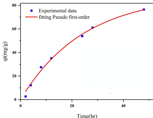
Fig. 11 Adsorption kinetics curve fit Pseudo 1st order model for Fe<sub>3</sub>O<sub>4</sub>@CS/UIO-66-NH<sub>2</sub>(Zr).
