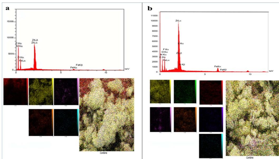
Fig. 5 EDX analysis and EDX elemental mapping of (a) Fe<sub>3</sub>O<sub>4</sub>@CS/UIO-66-NH<sub>2</sub>(Zr) and (b) PNT-Fe<sub>3</sub>O<sub>4</sub>@CS/UIO-66-NH<sub>2</sub>(Zr).
