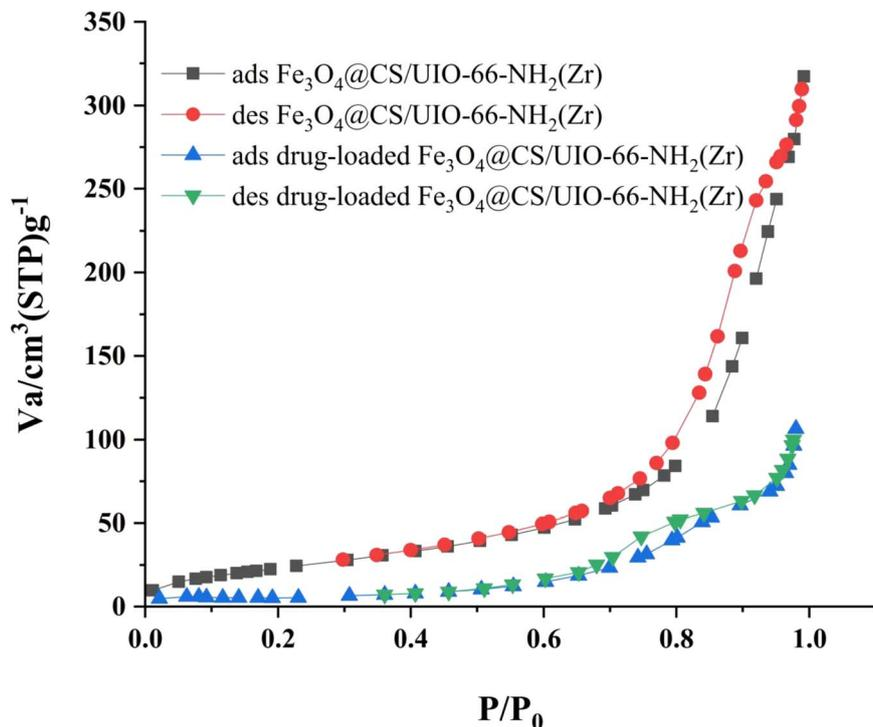
Fig. 7  $N_2$  adsorption–desorption  $Fe_3O_4@CS/UIO-66-NH_2(Zr)$  and drug-load  $Fe_3O_4@CS/UIO-66-NH_2(Zr)$ .
