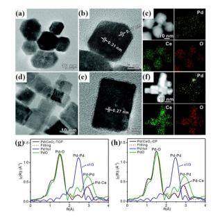
Fig. 7 (a) and (d) TEM and (b) and (e) HRTEM images of Pd/CeO<sub>2</sub>-TOP and Pd/CeO<sub>2</sub>-CP prepared via a photochemical route. (c) and (f) HAADF-STEM images of Pd/CeO<sub>2</sub>-TOP and Pd/CeO<sub>2</sub>-CP, and their corresponding EDX mappings of Pd, Ce, and O; Fourier transforms of EXAFS spectra for (g) Pd/CeO2-TOP and (h) Pd/CeO2-CP as well as the reference materials Pd foil and PdO at the Pd K-edge. Reproduced with permission. 33 Copyright 2017, The Royal Society of Chemistry.
