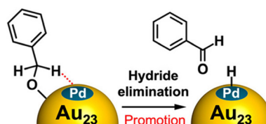
Fig. 2 Schematic illustration of the proposed mechanism by Pd doping on Au 24 :PVP. Reproduced from ref. 59 with permission from the American Chemical Society, Copyright 2022.
