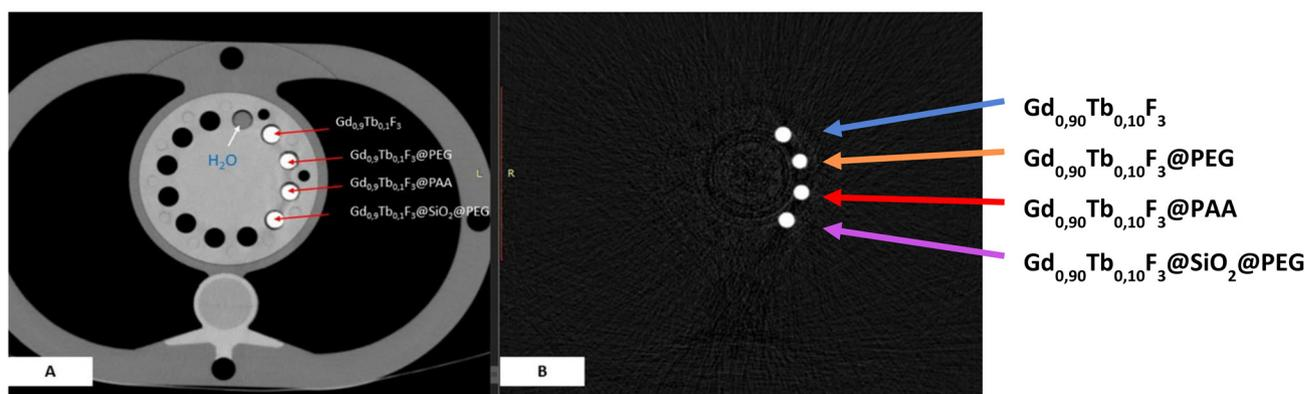
**Fig. 7** (A) Conventional SPCCT imaging of a phantom containing colloidal suspensions of normal, PEG modified, PAA modified and  $\text{SiO}_2@PEG$  modified NCs in water (0.5 M). (B) Same phantom with color gadolinium K-edge imaging using SPCCT.
