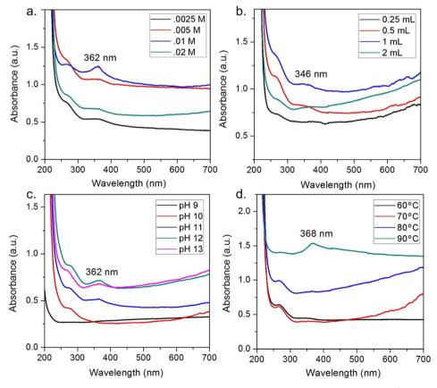
Fig. 6 Effect of factors on ZnO biosynthesis using *Nyctanthes arbor-tristis* floral extract, (a) concentration of  $Zn^{2+}$ , (b) volume of floral extract added into 50 mL of 0.01 M  $Zn^{2+}$  solution, (c) pH of the solution, (d) temperature of the solution. Reproduced with permission of Elsevier from ref. 59. Copyright 2018.
