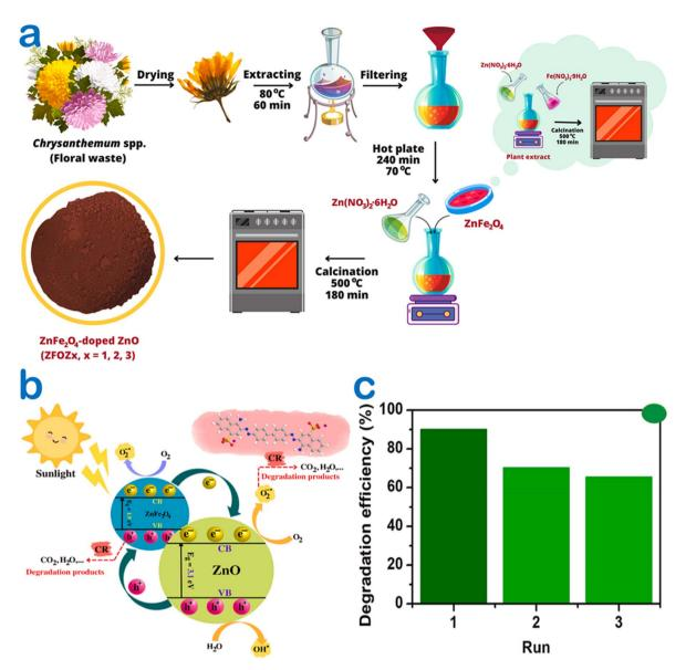
Fig. 8 (a) A schematic illustration of  $ZnFe_2O_4/ZnO$  nanocomposites biosynthesized using the *Chrysanthemum* spp. floral waste extract, (b) several plausible photocatalytic mechanisms under green  $ZnFe_2O_4$ -50%/ZnO catalysis for the degradation of the Congo red dye, (c) a recyclable run of  $ZnFe_2O_4$ -50%/ZnO for the degradation of the Congo red dye in the presence of solar light irradiation. Reproduced with permission of Elsevier from ref. 52. Copyright 2023.
