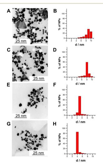
Fig. 3 TEM pictures and corresponding size distribution for CdSe NPs synthetized by chemical synthesis without apoferritin (A and B), chemical synthesis with apoferritin (C and D), electrochemical synthesis with apoferritin (E and F) and bioelectrochemical synthesis with apoferritin (G and H).
