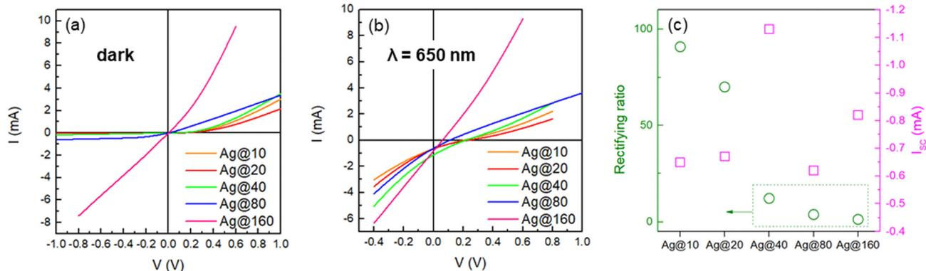
Fig. 4  $I$ - $V$  curves (a) in the dark and (b) under 650 nm wavelength laser light illumination with a fixed power density of  $877 \text{ mW cm}^{-2}$  for the different samples. (c) Rectifying ratio and short-circuit current achieved for the different samples.
