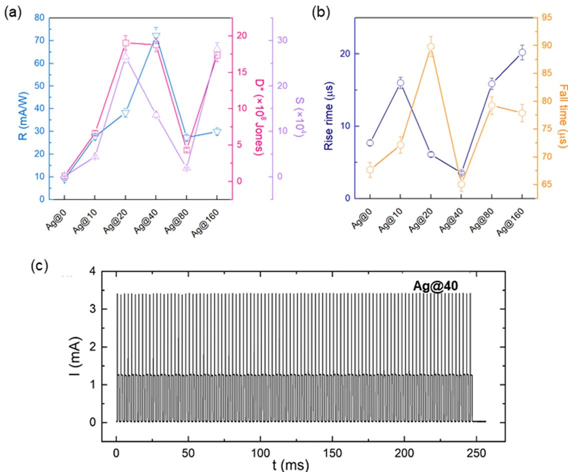
Fig. 7 (a) Responsivity ( $R$ ), detectivity ( $D^*$ ) and sensitivity ( $S$ ) for the different samples. (b) Rise time ( $\tau_r$ ) and the fall time ( $\tau_f$ ) estimated for the different samples. (c) Stability of the transient response characteristics of the Ag@40 sample under zero bias and with 650 nm laser illumination and a laser power density of  $887 \text{ mW cm}^{-2}$ .
