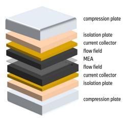
Fig. 9 Visualization of the cell setup.
