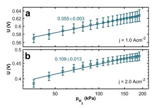
Fig. 3 Logarithmic plot of the voltage at a current density of (a) 1.0 A cm<sup>-2</sup> and (b) 2.0 A cm<sup>-2</sup> against the hydrogen partial pressure. The lines serve as a guide for the eye.
