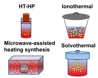
Fig. 2 Schematic diagram of synthesis method: high temperaturehigh pressure method, ionothermal route, microwave-assisted heating synthesis, and solvothermal approach.
