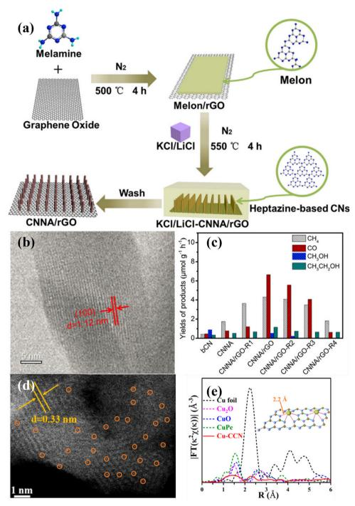
Fig. 17 (a) Schematical illustration of the preparation of CNNA/rGO. (b) HRTEM image of CN nanorod in CNNA/rGO. (c) Photocatalytic CO<sub>2</sub> reduction activities of bCN, CNNA, CNNA/rGO-R4, and CNNA/rGO. Reproduced with permission: 175 Copyright 2019, Elsevier. (d) HAADF-STEM image of Cu-CCN. (e) FT-EXAFS of the samples. 184 Copyright 2020, American Chemical Society
