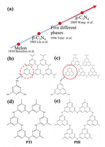
(a) The roadmap of the development of carbon nitrides. (b) Triazine and (c) tri-s-triazine (heptazine) structures of g-C<sub>3</sub>N<sub>4</sub>. (d) Structures of poly(triazine imide) (PTI) and (e) poly(heptazine imide) (PHI).
