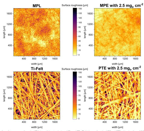
Surface distance maps from the XTM data of the stand-alone MPL and PTL (Ti-felt) as well as the MPE and PTE with a loading of 2.5 mg<sub>lr</sub> cm<sup>-2</sup>.
