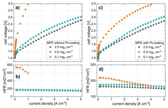
Fig. 7 Polarization curves and HFR measurements of cells with an MPE approach at the different iridium loadings (N115, T = 80 °C, 10 bar balanced pressure) using MPLs (a) and (b) without Pt-coatings and (c) and (d) with a Pt-coating (40 nm).
