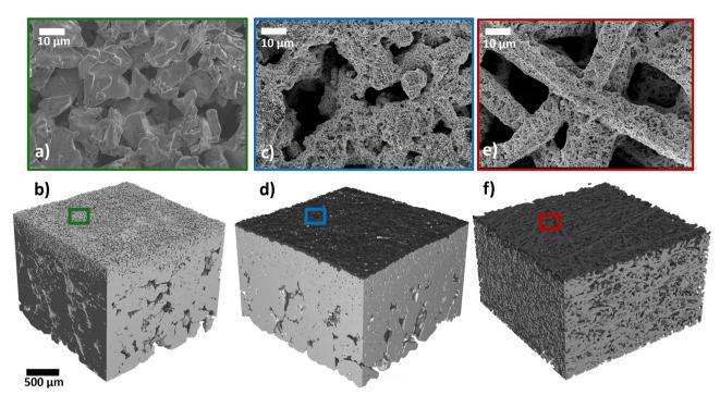
Fig. 3 (a), (c) and (e) Top view SEM images and (b), (d) and (f) XTM surface renderings of (a) and (b) MPL + support layer; (b) and (d) MPE with 2.5 mg<sub>lr</sub> cm<sup>-2</sup> loading; and (e) and (f) Ti-felt (Bekaert) with 2.5 mg<sub>lr</sub> cm<sup>-2</sup>.
