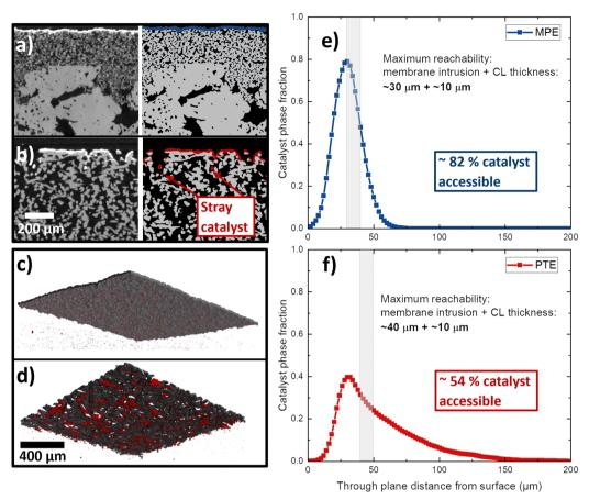
Fig. 4 Cross-section XTM slices, as grey-scale and segmented images of (a) an MPE and (b) a PTE (based on Ti-felt) with 2.5 mg<sub>Ir</sub> cm<sup>-2</sup> catalyst layers. Three-dimensional visualization of the catalyst layer for (c) the MPE and (c) PTE where the voxels in the CL that are part of the continuous network are shown in black, whereas the isolated voxels are visualized in red. Catalyst layer phase fraction distribution across the thickness of (d) PTE and (e) MPE.
