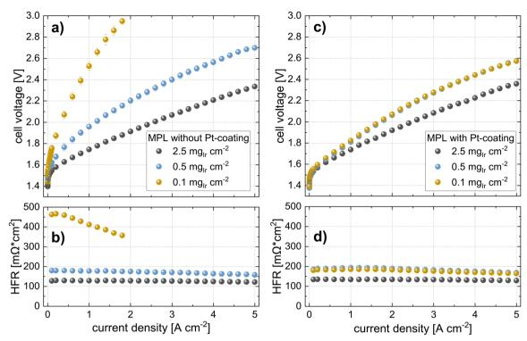
Fig. 6 Polarization curves and HFR measurements of cells with a CCM (N115) approach at the different iridium loadings (T = 80 °C, 10 bar balanced pressure) using MPLs (a) and (b) without Pt-coatings and (c) and (d) with Pt-coating (40 nm).
