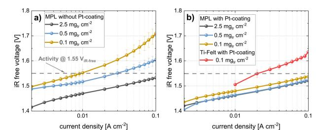
Fig. 9 Semi-logarithmic plots of the iR-free cell voltage vs. current density (Tafel-plots) for all loadings in CCM configuration (a) MPLs without Ptcoating (b) MPLs with Pt-coating and comparison with Ti-felt reference with Pt-coating; all measurements with N115, at T = 80 °C and 10 bar balanced
