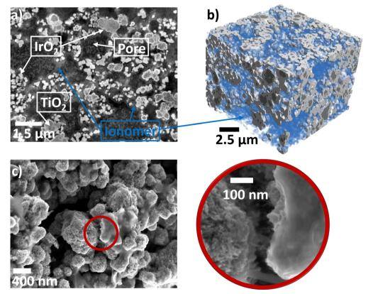
Fig. 1 (a) Grey-scale slice of the CL (dry) extracted from the 3D volume obtained by PyXL (b) surface rendering of the volume with the ionomer phase shown in blue (c) SEM images of the CL particles and ionomer layer at two magnifications.
