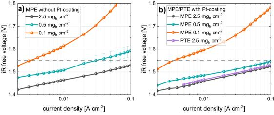
Fig. 10 Semi-logarithmic plots of the iR-free cell voltage vs. current density (Tafel-plots) for all loadings in MPE configuration (a) MPLs without Pt-coating, (b) MPLs with Pt-coating and comparison with Ti-felt reference (PTE with Pt-coating); all measurements with N115, at T = 80 °C and 10 bar balanced pressure.
