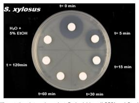
Fig. 9 Toxicity test for untreated (t = 0) and treated water collected at different time intervals against Escherichia coli SCS1 and Staphylococcus xvlosus.
