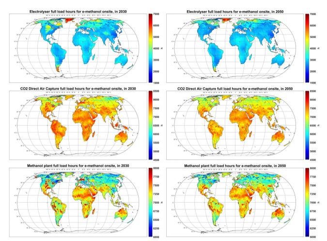
Full load hours of electrolyser (top), CO<sub>2</sub> direct air capture (centre) and methanol plant (bottom) in 2030 (left) and 2050 (right)
