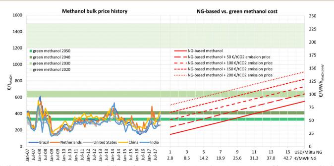
Fig. 12 History of methanol bulk market prices (left) and NG-based vs. green methanol cost for varying natural gas and CO<sub>2</sub> emission prices (right). Green methanol cost range at best sites with 20  $Gt_{MeOH}$  per year cumulative production potential. Methanol price history is based on data from Intratec<sup>65</sup> and a 1.2 € per USD exchange rate.
