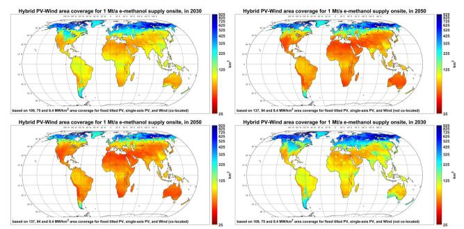
Fig. 8 Area coverage of hybrid PV-wind power plants for 1 Mt per year e-methanol supply in 2030 (left) and 2050 (right) with PV and wind plants not colocated (ton) and co-located (bottom)
