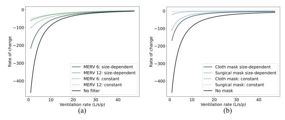
Fig. 5 Rate of change of virus concentration with ventilation for long-range airborne transmission when with constant and size-dependent efficiency of filters/masks and when without filters/masks. (a) Ventilation-filtration; (b) ventilation-mask.
