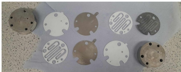
Fig. 2 Electrochemical flow reactor components. 2× stainless steel (SS) electrodes and 1× graphite electrode. 2 PTFE spacers (1 mm thickness) were used, each with a flow channel volume of 0.464 mL. This gave an overall reactor volume of 0.928 mL.
