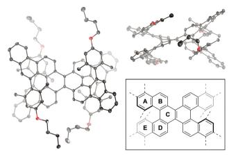
Fig. 2 X-ray crystal structure of  ${\bf 1}$  with thermal ellipsoids at 50% probability; all hydrogen atoms are omitted for clarity. Inset: definition of rings A-E.
