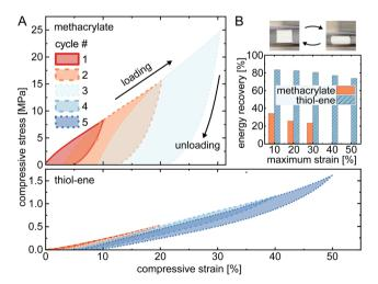
Fig. 2 Comparative cyclic compressibility and energy recovery. (A) Cyclic compressibility of a porous thiol-ene and methacrylate-based material. (B) Energy recovery calculated for both materials using the ratio between the areas under the unloading and loading curves.
