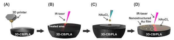
Fig. 1 Scheme of the 3D-printed electrode fabrication and modification steps: (A) printing, (B) IR-laser ablation, (C) drop-casting, and (D) IR-laser modification of 3D-CB/PLA.
