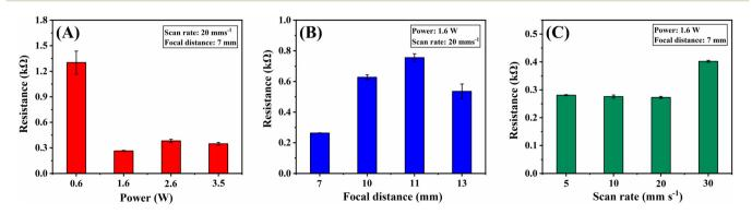
Fig. 2 Effect of IR-laser parameters variation on the electrical resistance of treated 3D-CB/PLA electrodes: (A) IR-laser power (W), (B) focal distance (mm), and (C) beam scan rate (mm s<sup>-1</sup>).
