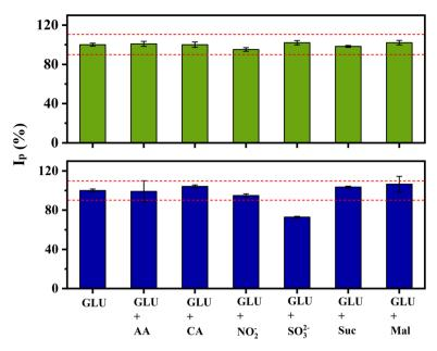
Fig. 7 Interference study performed by LSV with 1.0 mmol L<sup>-1</sup> glucose (Glu) in the presence of 0.1 mmol L<sup>-1</sup> (green bars) and 0.5 mmol L<sup>-1</sup> (blue bars) of ascorbic acid (AA), citric acid (CA), nitrite (NO<sub>2</sub><sup>-</sup>), sulphite (SO<sub>3</sub><sup>2</sup><sup>-</sup>), sucrose (Suc) and maltose (Mal). The values correspond to the average of three measurements (n = 3).
