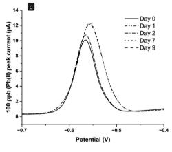
Fig. 6 (a) SWASV signal of a 0.1 M HCl solution containing 100 ppb Pb (ii) on Day 3 using an external Ag/AgCl reference electrode. (b) Peak heights and (c) voltammograms obtained for 100 ppb Pb(ii) using 0.1 M acetate buffer (pH 4.75) as medium to study the stability of the flow system during consecutive days; the bars represent average peak currents resulting from SWASV (n=6 per day, total number of measurements: 54); the potentials are referred to the external Ag/AgCl reference electrode.
