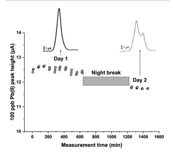
Fig. 5 Stability of the modified sensors during a two days measurement session for the detection of 100 ppb Pb( $_{\rm II}$ ) in 0.1 M HCl; measurements were performed every hour in triplicate (except for a 10 hour night break) for a total of 42 scans. The scans above show the peak splitting phenomenon: comparison between the SWASV signal obtained on the first scan of Day 1 and that on Day 2.
