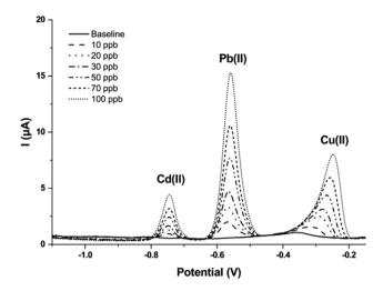
Fig. 7 SWASV scans obtained for Cd(II), Pb(III), and Cu(III) in the range 0–100 ppb under optimized conditions; the measurements were performed using 0.1 M acetate buffer (pH 4.75) as medium.
