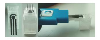
Fig. 6 Three-dimensional printed case for the integration of the printed electrode and alginate spheres.
