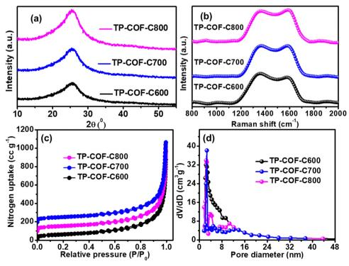
Fig. 2 (a) PXRD pattern and (b) Raman spectra of TP-COF-C samples. (c) Nitrogen adsorption—desorption isotherm and (d) the corresponding pore size distribution plot of all the TP-COF-C samples.
