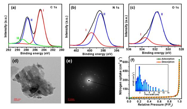
Fig. 1 Core level XPS spectra for (a) C 1s, (b) N 1s, and (c) O 1s of TP-COF. (d) TEM images and (e) corresponding SEAD image of TP-COF. (f) N<sub>2</sub> adsorption-desorption analysis of TP-COF and the corresponding pore size distribution plot of TP-COF in the inset
