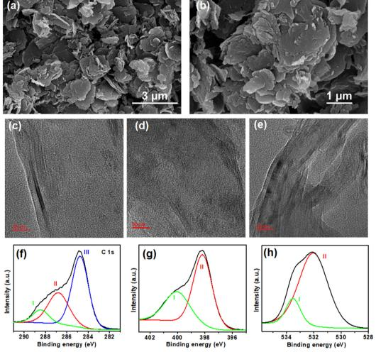
Fig. 3 (a) and (b) The SEM images of TP-COF-C700 in different resolutions. The HRTEM images of (c) TP-COF-C600, (d) TP-COF-C700, and (e) TP-COF-C700 in different resolutions. COF-C800. The core-level XPS spectra of (f) C 1s, (g) N 1s, and (h) O 1s of TP-COF-C700
