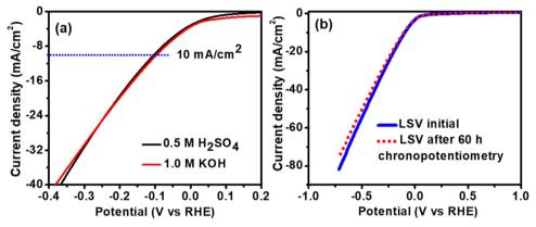
Fig. 5 (a) The LSV curves of TP-COF-C700 using 0.5 M H $_2$ SO $_4$  (black line) and 1.0 M KOH (red line) electrolytes. (b) The LSV polarization curves of TP-COF-C700 before and after 60 h chronopotentiometry using 1 M KOH as electrolyte.
