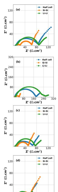
Fig. 1 EIS spectra collected for comparison between half cells and symmetric cells at (a) 0.2 V in the lithiation step; (b) 0.07 V in the lithiation step; (c) 0.3 V in the delithiation step; (d) 0.48 V in the delithiation step.
