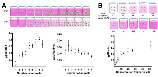
Fig. 1 Optimization of animal number (A) and concentration of microparticle (B) in the feeding assay. (A) One to nine animals were incubated in 6 ml of microparticle at a final concentration of 13 mg l<sup>-1</sup>. (B) Six animals were incubated in 6 ml of different concentrations of microparticle (1.3 to 52 mg l<sup>-1</sup>). Data represent average  $\pm$  standard deviation (N = 4).
