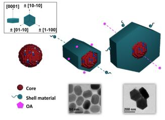
Fig. 2 Proposed mechanism of epitaxial growth of NaLnF<sub>4</sub> shells around the NaYbF<sub>4</sub>:Tm(0.5%) Fe(5%) core.
