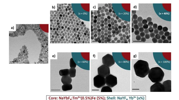
Fig. 1 TEM images of core and core@shell structures using different Yb<sup>3+</sup> concentrations during shell growth. (a) NaYbF<sub>4</sub>:Tm(0.5%) Fe(5%) core and (b)-(g) NaYbF<sub>4</sub>:Tm(0.5%) Fe(5%)@NaYF<sub>4</sub>:Yb(x%)-core@shell where x = 0%, 20%, 40%, 60%, 80%, and 100%. Size histograms are shown in Fig. S1 (ESI†). All scale bars show 100 nm.
