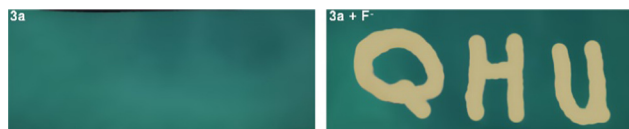
Fig. 5 The 3a based film sensors for fluoride anions under UV irradiation ( \lambda_{\text{ex}} = 365 nm).
