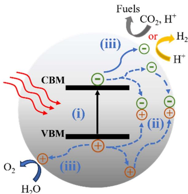
Fig. 3 Scheme of the photocatalytic  $\text{CO}_2$  reduction reaction and water splitting for the semiconductor. CBM: conduction-band minimum; VBM: valence-band maximum. (i) Absorption of photons. (ii) Charge separation, migration and recombination. (iii) Surface reactions.
