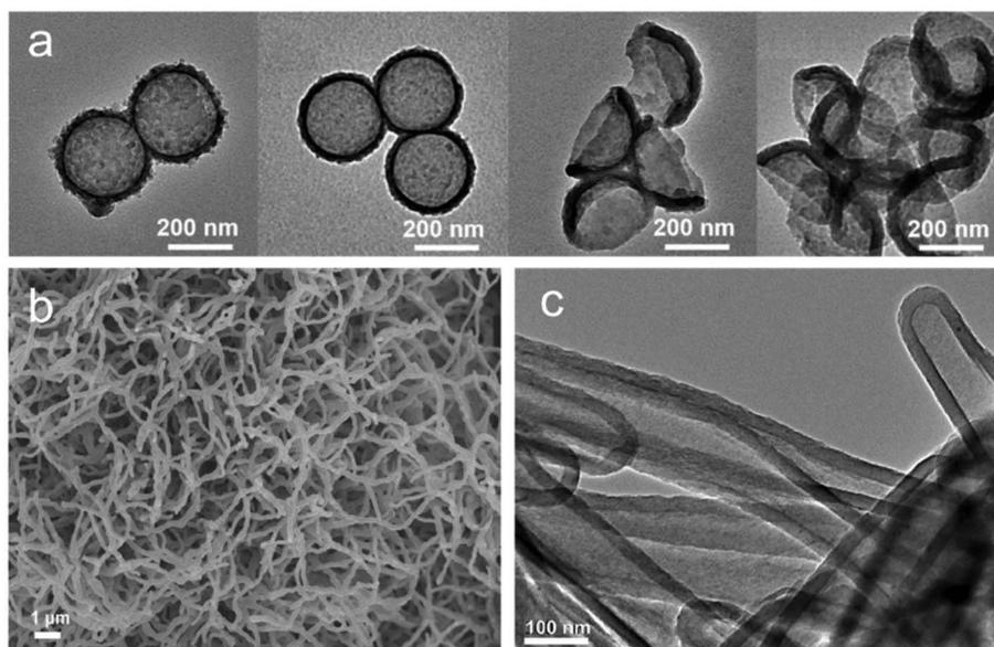
Fig. 12 (a) The transmission electron microscope (TEM) images of different etched CTFs. Reproduced with permission from ref. 136. Copyright 2019, John Wiley and sons. (b) SEM and (c) TEM images of olefin-linked CTF nanotubes. Reproduced with permission from ref. 71. Copyright 2021, Elsevier.
