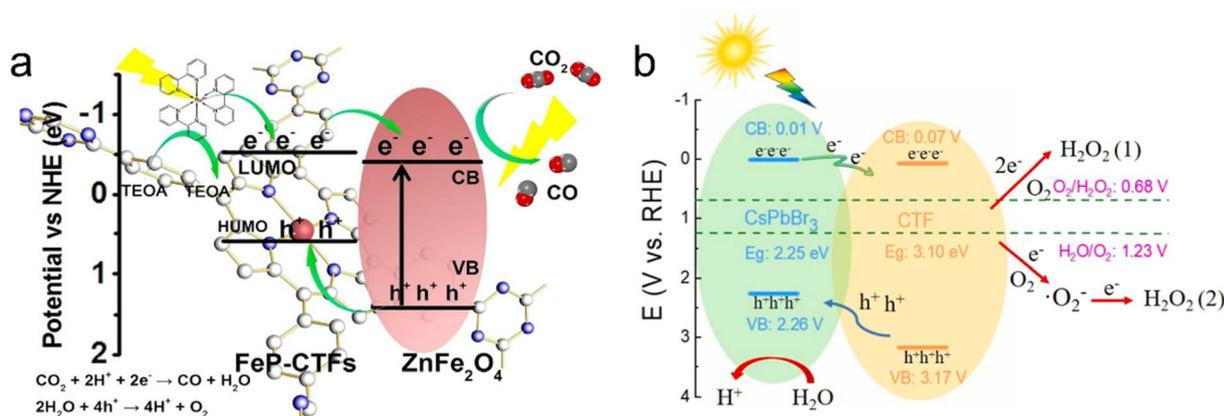
Fig. 16 The proposed charge transfer mechanisms: (a) ZnFe<sub>2</sub>O<sub>4</sub>/FeP-CTF for the photocatalytic CO<sub>2</sub> reduction system. Reproduced with permission from ref. 183. Copyright 2021, Elsevier. (b) CsPbBr<sub>3</sub>/CTF-2 for photocatalytic H<sub>2</sub>O<sub>2</sub> production. Reproduced with permission from ref. 186. Copyright 2022, Elsevier.
