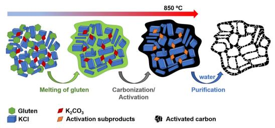
Scheme 2 Experimental procedure used for the synthesis of AGA-850.
