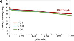
Fig. 7 (a) Ragone plot showing the energy/power performance of the NICs and (b) long-term cycling test performed at 2 A  $g^{-1}$ .
