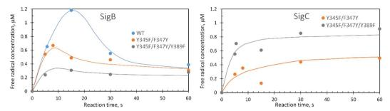
Fig. 7 Comparison of SigB and SigC formation for the double and triple DtpAa variants. Plots represent the first 60 s of the EPR time course following a 10-fold addition of  $H_2O_2$  to a 40  $\mu$ M DtpAa sample. The solid lines through the data points are to guide the eye.
