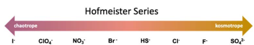
Fig. 3 Common anions in the Hofmeister series. This represents a common reference framework for electrochemical sensors. Electrochemical sensors are commonly more sensitive to charge diffuse chaotropes (left) than charge dense kosmotropes (right). In this study, we place \text{HS}^- in the series between \text{Cl}^- and \text{Br}^- ( vide infra ).
